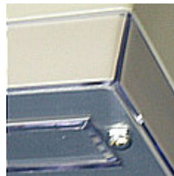
Aluminum sheet & acrylic front panel
