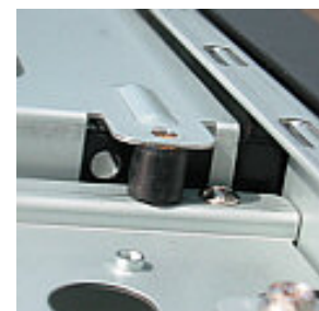
Drive cage rubber grommets
