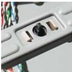
Intruder alarm on top bar
