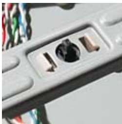
Intruder alarm on top bar
