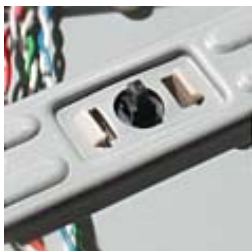
Intruder alarm on top bar
