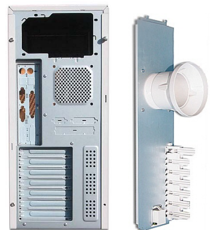
Back view & Metal bar With air duct and card holders.
